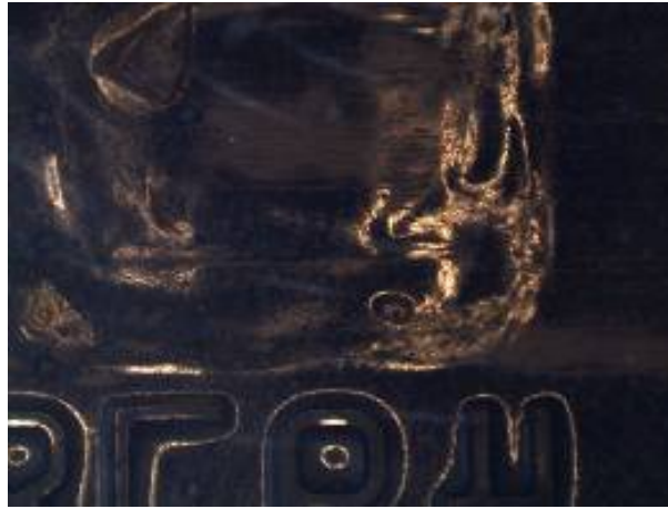
Figure 5.14 – Deformation due to heating of the forgery's backside.
