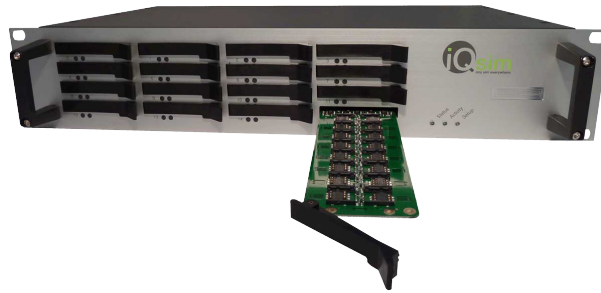
Figure 5.33 – An industrial multi-SIM reader.
