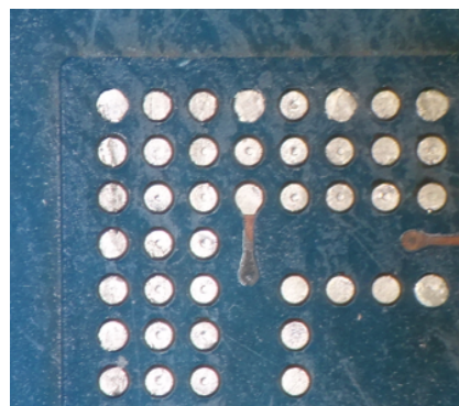
Figure 7.10: Donor Board eMMC Gap Position
