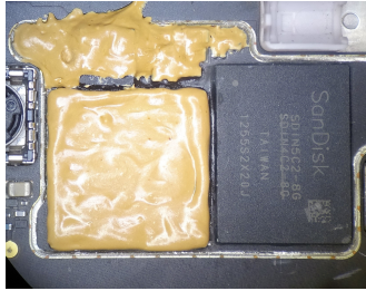
(a) Protecting the Donor Board With Adhesive
