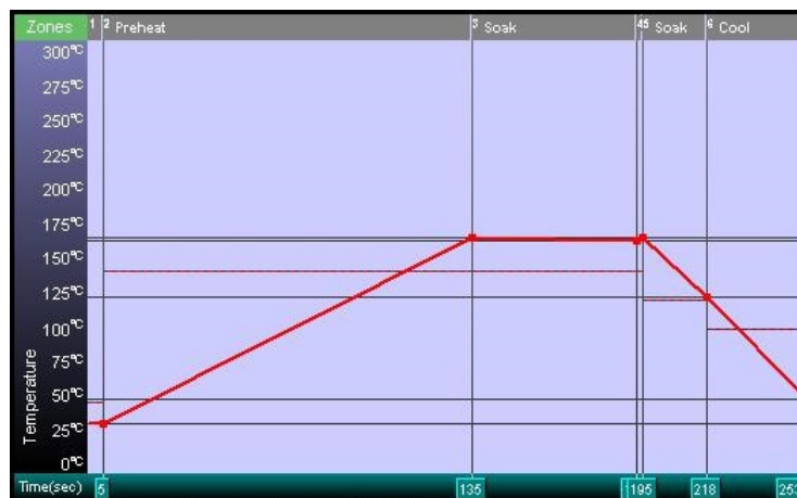
Figure 4.26: Fast Cooling (1.9 °C/s) Reflow Profile, X-axis (seconds), Y-axis (Celsius)
